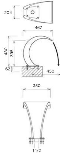
**ANCLAJE CASCADA MINI BALI • ANCHOR FOR WATER CURTAIN MINI BALI • ANCRAGE POUR CASCADE MINI BALI**
