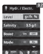
9.2 Level: Hydrolysis - Desired disinfection production (Always 100%).
