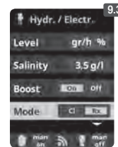
9.3 Mode: If the device has Free Chlorine and redox probes, choose the parameter that controls the cell's chlorine generation.
